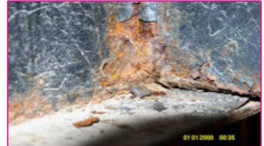
vehicle created a disproportional weight condition. Generally the cause is a corroded frame that has lost some of its structural strength, or it has been subjected to greater loads than it can now carry. Only in rare occasions have the manufacturers been responsible for frame failures. In those instances thin frames with multiple slide-outs were most prevalent.
