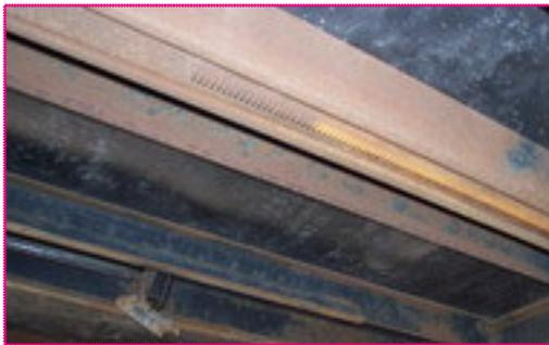
upon an RV frame and those loads are subjected to forces greater than the stand-alone area of design, it will flex, twist, bend and then normally return to the original designed shape. The degree of flex before the metal fractures depends upon many factors. Some are temperature, hardness of the metal and the plus and minus loads exerted (up and downward movement while driving on the highway). When frames fail it is generally due to an under design, fatigue, impact damage, corrosion, or
